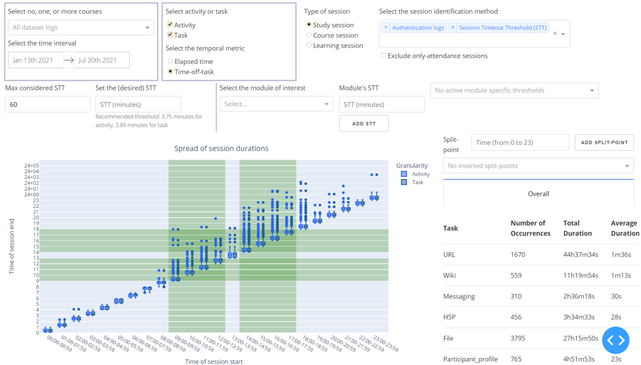
Figure 4. Visual tool’s appearance. The top panel allows the user to pick data and parameters, while the bottom panel displays the plot used to define the time-windows on the left and the table on the right displays information on the occurrences of ending modules overall and for each manually inserted time-window.
