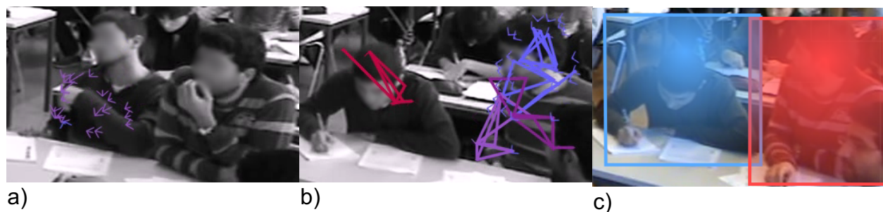
Figure 2: Motion detection and grouping. a) Individual motion vectors shown as purple arrows, b) motion vectors grouped over time into motion tracks that can be assigned to an individual, and c) marked student areas and centres of Gaussian probabilities, which model the probability of motion belonging to each student.
